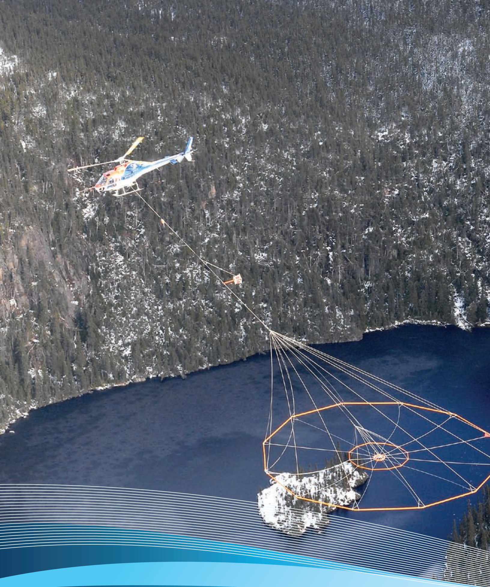
Helicopter carrying electromagnetic survey equipment
